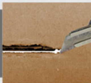
Poor cut line
